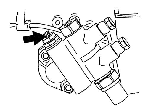
CHECKING AND ADJUSTING TIMING-DEVICE PROFILE
